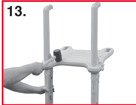
13. Stand the ladder up, using a rubber mallet tap the platform down until seated on the lugs on the ladder leg. IT WILL REQUIRE SEVERAL HARD BLOWS WITH A RUBBER Mallet TO SEAT THE PLATFORM ALL THE WAY DOWN ONTO LUGS.
